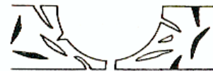
Make use of a gouging electrode to make a groove and at same time burn out the oil
