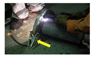
Try to place the return clamp as close to the cut line as possible. If possible, place the clamp on the workpiece itself. Inspect the cables for loose connections, worn spots, or anything else that might resist the electrical flow. Only secure the return clamp to clean metal for getting the best cutting performance. Grind off the paint or rust before clamping as these may inhibit the flow of electricity.
