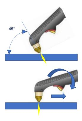
Pierce cuts are a little more difficult. The torch will need to be angled slightly over the starting point. This will prevent the molten metal from the beginning of the cut from being blown back into the tip and electrode.
