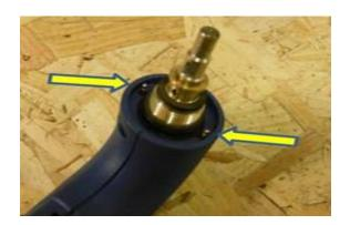
Note safety pins that break the circuit in the moment the shield cup is removed.
