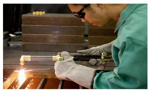
Why is it that we only can use the flame cutting processes on steel? In order for a metal to be cut by flame (oxy-acetylene/ oxy-propane) the following must apply:
