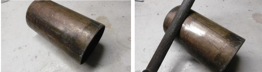
A Yorcalbro seawater pipe, yellowish brown surface. Freshly filed relives a silvery yellow.
