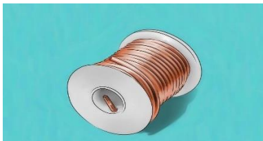
Soft solder on roll with or without ducts filled with flux (flux core)
