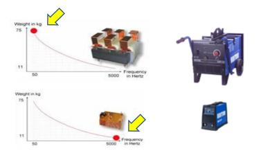
Note the dramatic weight reduction when we go from Rectifier to Inverter technology. The Rectifier deliver 300 Amp and have a weight of 95Kg The Inverter deliver also 300 Amp and have a weight of only 18Kg.
