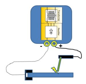
Rectifiers have a transformer part that brings high voltage to low voltage and in addition a rectifier part that convert Alternating Current to Direct Current. The direction of the electrons is from - to +.
