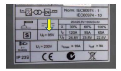
This is the motor plate on a land-based welding machine. It has CE, S, IP 23S so all looks good except for OCV that is far above legal limit for use on-board.
