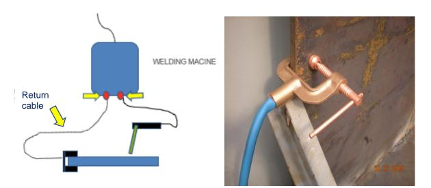
The return cable on an arc welding machine carries just as much current as the welding cable itself. Both the welding and return cables are part of the electric circuit. As a result, for safe welding the welder must use a return clamp and cable, which must be placed as near to where the welding is taking place as possible.
