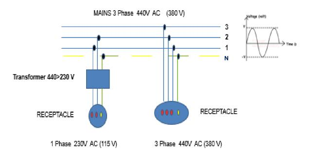
Usually a ship's electrical distribution scheme follows shore practice. This allows normal industrial equipment to be used after being adapted and certified where and if necessary, so it can withstand the conditions on board a ship (e.g. vibration, freezing and tropical temperatures, humidity, the salty atmosphere, etc. encountered in various parts of the ship).
