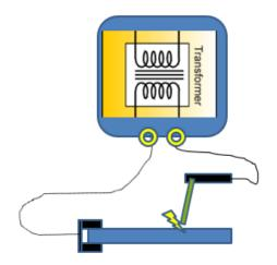
Transformers consist of an iron frame with primary and secondary copper windings. The current from the mains entering the primary windings create a magnetic field in the iron frame that are picked up by the secondary windings. An iron core regulated by a crank can be lowered or hoisted inside the frame to create alterations in Amperage. You recognize Transformers because of a hand crank on front or top and no +/- signs on the terminals (machine front).
