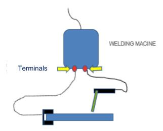
Receptacles for 1 phase 230V AC (sometimes 115V AC) are to be found at most locations onboard. If the receptacle delivers 230V and is fitted with 16 Amp slow fuse it will be able to power smaller welding machines that can deliver up to 150 Amp. If 115V the welding machine might deliver approximately 95 Amp. Receptacles for 3 phase 440V AC (sometimes 380V AC) can sometime be more limited onboard and are used for bigger size welding machines.
