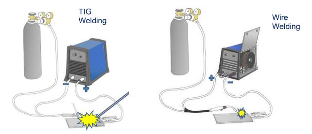
Wire Welding is a process where a wire from a reel is fed through a welding torch passing a contact tip supplying the welding current. The wire melts and is transferred to the pool through the arc. A shielding gas is in most cases necessary to prevent air oxidising the pool. The process can roughly be divided into two distinctive methods:
